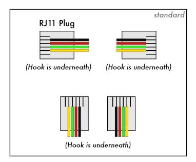
This is often mistaken as "straight-through", mainly due to fact that if you were to stretch the cable out, the wires would stay side by side the whole length without going over each other. This, however, is incorrect.
