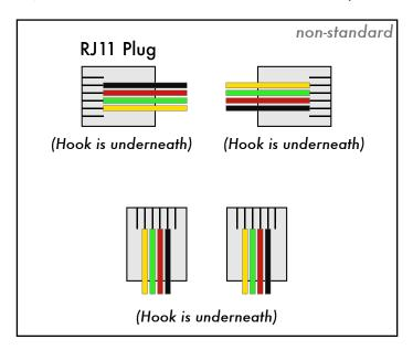
When it is "reverse," however, the wires are mirrored (as shown below).
