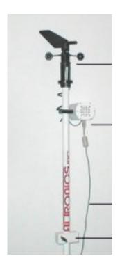
Face mark on Wind Sensor housing towards finish line (parallel to race track)
